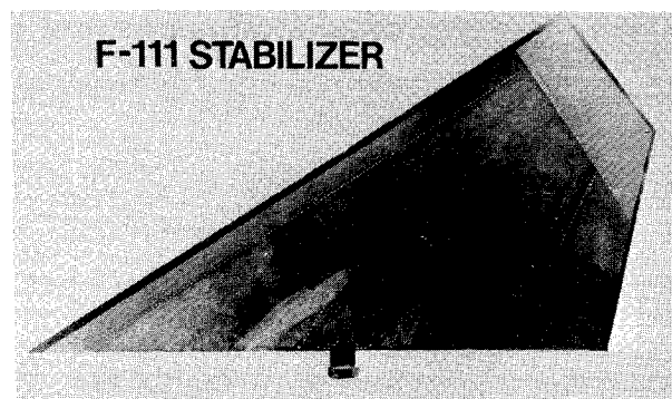
Fig. 10 The first generation advanced composites component was demonstrated by the F-111 horizontal stabilizer. This item achieved the objectives of technology demonstration in terms of materials, design, and manufacturing. This empennage technology was readily transferred from General Dynamics to other aerospace companies.
